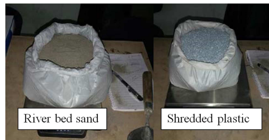
Figure 7. Proportioning of plastic and sand.
