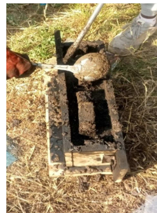
Figure 11. Casting the mixed plastic and sand.
