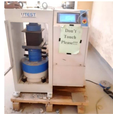
Figure 13. Compressive strength test by UTM.
