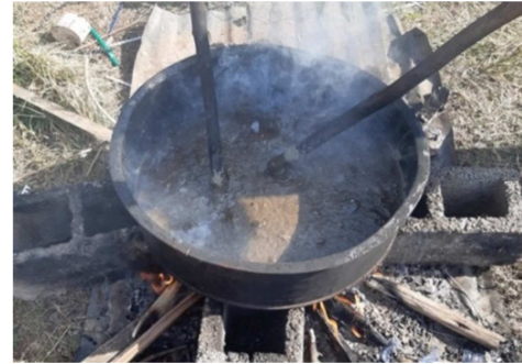
Figure 10. Melting the plastic (HDPE & PET) to mix with sand.
